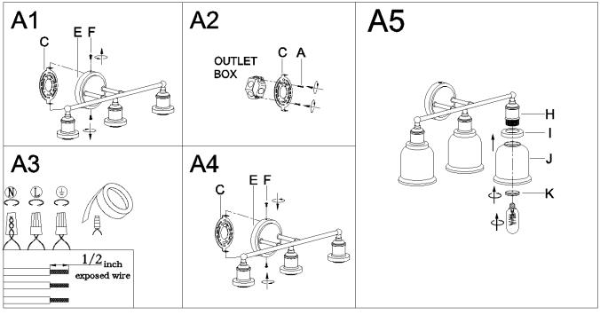
Step A1: Unscrew the grub screw (F) from the back plate (E) then gently remove the mounting plate (C). Step A2: Secure mounting plate (C) to outlet box with mounting screws (A). Step A3: Make wire connections
