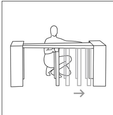
Hide the center leg when using less than two panels.
