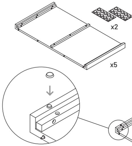
Each Transformer Table comes with a package of 2 protective pads you will need to install onto each panel to prevent damage when they are being stored.
