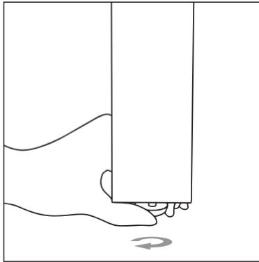
Adjust the middle leg to level the height of the table.
