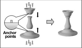
Assemble the 3 parts of the holder into a hole with 8 screws. **Note:** Be sure to have the corresponding anchor points lined up correctly before fixing.
