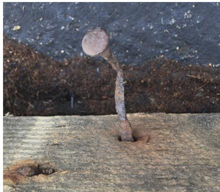
The effect of corrosion on HDG spikes.
