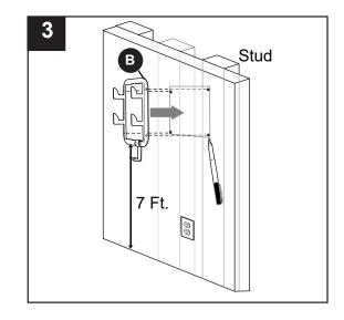
Use 3/32-in. drill bit (not included) to drill pilot holes at marked locations. Then, install wall mounting bracket (B) to mounting surface with wood screws (AA).
