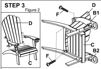
Attach back support (D) onto the assembly from step 2 as figure 2.
