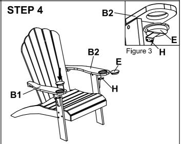
Attach the wooden plug (E) onto armrest (B1&B2). "The wooden plug can be used as base for drinkware, as shown in figure 3".
