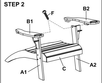
Attach the armrest (B1&B2) onto the legs (A1&A2), secure using 1" bolts (F).
