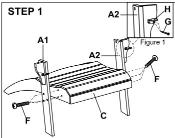
Attach right and left leg (A1&A2) to seat (C). Secure with 1" bolts (F).
