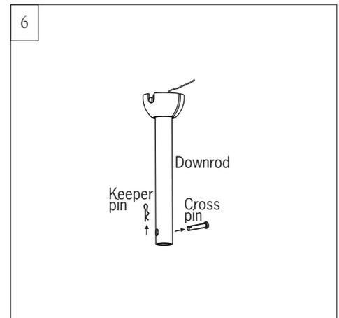
Remove preassembled cross pin and keeper pin from downrod. Keep parts.
