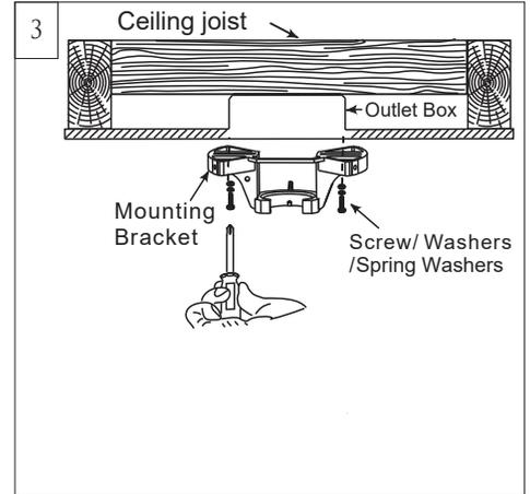
Use metal outlet box suitable for fan support and use only the screws provided with the outlet box (must support 35 lbs). Remove the two outlet box screws provided with the box, aligning the holes of the mounting bracket with the holes of the outlet box. Reinstall the 2 outlet box screws securely.
