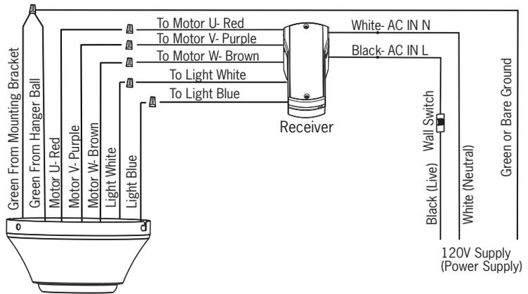
Make wiring connections using wire connectors provided as indicated above.
