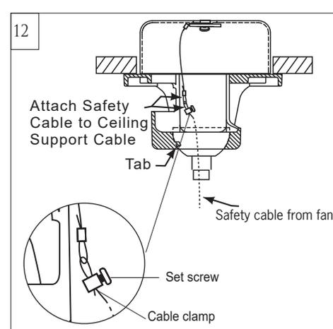
Connect the safety cable from fan to the Ceiling support cable. Slide cable clamp onto the safety cable from fan. Place the end of cable through the loop of ceiling support cable and then feed end of cable into clamp hole and firmly tighten set screw. Cut off excess safety cable. Make sure that when the safety cable is fully extended the lead wires are longer than the cable and no stress is placed on the lead wires.
