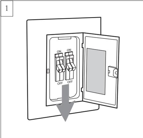
Before you begin installing the fan, Switch power off at Service panel and lock service disconnecting means to prevent power from being switched on accidentally. When the service disconnecting means cannot be locked, securely fasten a warning device, such as a tag, to the service panel.
