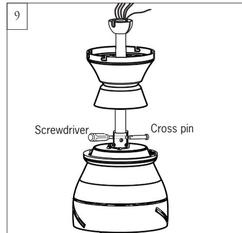
For easy installation of cross pin on next step. Carefully insert a phillips screwdriver through yoke and downrod (don't damage the lead wires) as a guide and then push the cross pin and pull the screwdriver in the meantime as shown in illustration.
