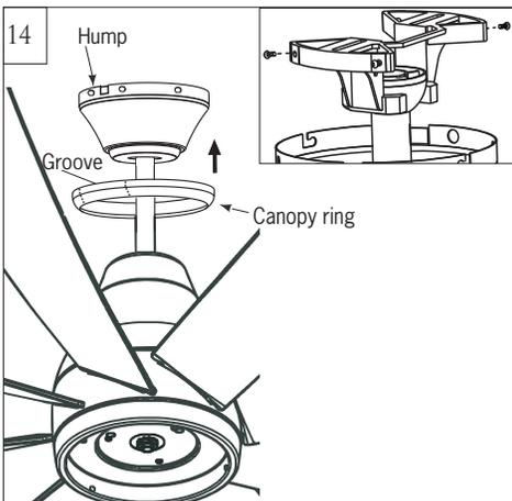
Partially loosen 2 of the set screws on mounting bracket corresponding to the slotted holes on the canopy upper ring. Remove the other 2 set screws. Save screws. Raise canopy to mounting bracket, aligning loosened screws in mounting bracket with slotted holes in canopy. Twist canopy clockwise to lock. Reinstall the screws just removed and then tighten all screw securely. Install canopy ring onto canopy by aligning the grooves in canopy ring with the humps on canopy and snap it onto canopy.
