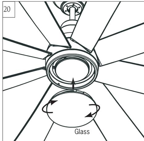
Attach glass to light pan by locating dimples in light pan with grooves in glass and twist clockwise until tight.
