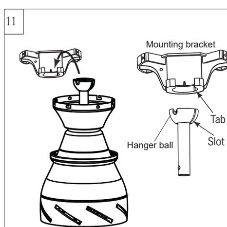
Install ball end of downrod into mounting bracket opening. Align (engage) slot on ball with tab on mounting bracket. **Warning:** Failure to align slot on ball with tab may result in serious injury. **Important:** If using the angle mount, make sure open end of mounting bracket is installed facing the higher point of the ceiling and make sure the ceiling angle is not steeper than 15°.
