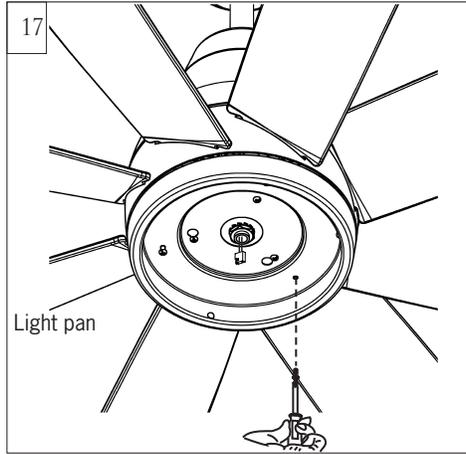
Loosen 2 and remove 1 preassembled screw from the light pan. Save screws for later use.
