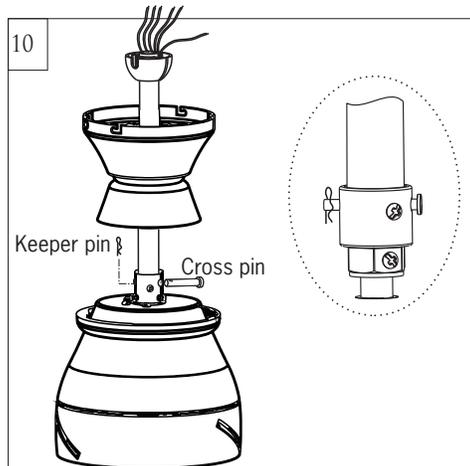
Slip downrod into motor yoke, aligning holes and install cross pin and keeper pin. Insert cross pin through yoke and downrod until point appears on the other side, and insert keeper pin on cross pin. Pull the downrod up tight against the cross pin, and then evenly tighten the downrod set screws on motor housing yoke. Place yoke cover on top housing of fan. **Warning:** Cross pin and keeper pin must be installed securely, failure to install them will result in serious injury.
