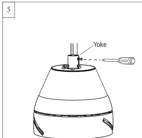
Partially loosen downrod set screws from yoke at top of motor assembly.
