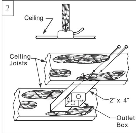
Before installing this fan make sure the outlet box is properly installed to the house structure. Ensure the outlet box is securely fastened by at least two points to a structural ceiling member (a loose box will cause the fan to wobble). To reduce the risk of fire, electric shock, or personal injury, mount to outlet box or supporting system acceptable for fan support. (Mounting must support at least 35 lbs.)
