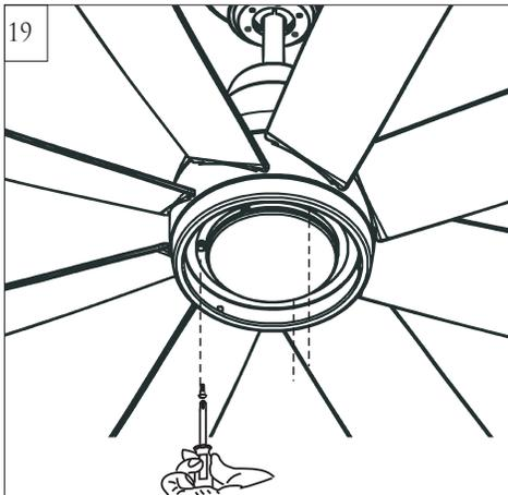
Attach LED light fixture onto the light pan, aligning the keyhole slots on the LED light fixture with the preassembled screws on the light pan. Twist clockwise till lock. Reinstall the screw removed in step 17. Tighten all screws securely.
