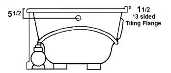
Standard (S) Pump Location \*\*Skirt access is very limited Additional side access is recommended
