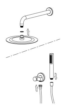
6. Install shower arm and hand shower bracket (wrap the PTFE tape on the thread).
