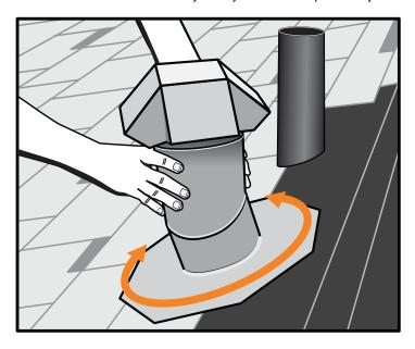
1. Set **TOTAL JACK™** down, flat on the surface of the roof, next to the pipe you are ventilating. Rotate the octagonal base flange to achieve a vertical, upright position.
