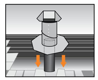
2. Place TOTAL JACK™ over the pipe (a). Adjust base, if necessary.
