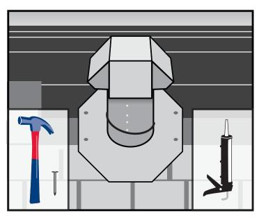
**3**. Secure octagonal flange with fasteners as approved by your local building code. Add a dab of caulking to seal the fasteners Install remaining shingles in accordance with manufacturer's specification.
