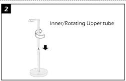
Place the outer/lower end of the tubing sub-assembly onto the bolt at the top of the Insert bolt on pivot arm sub-assembly into top of tubing. Hold the inner/upper base. Hold the outer/lower tube and turn clockwise to fasten the tubing onto the base. Hand tighten only.
