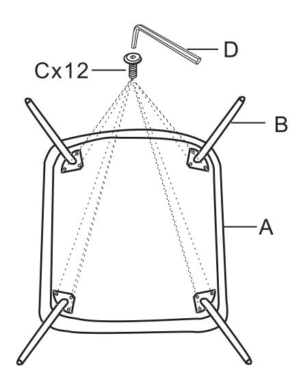
**STEP 3 :** Use bolt C, allen key D to connect the metal leg B to bottom of the seat cushion A, make sure all holes algin, fasten all bolts to secure.
