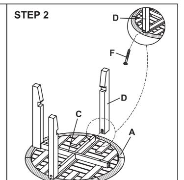
Next, attach three legs (D) into pre-assembled. Secure with 2" bolts (F). Do not fully tighten all bolts yet.
