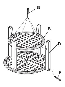
Attach the tray (B) into three legs (D) secure using 1 1/2" screws (G). Next, attach the remaining leg (D) into tray (B) and apron (C), secure using 2" bolt (F). Fully tighten all bolts and screws.
