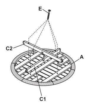
Attach Upper and Bottom Apron (C1 & C2) into top table (A). Secure with 1 3/4" bolts (E)
