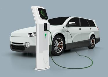
When charging the EV battery, charging occurs at the full rate until the battery approaches 80%. At that point, the rate of charging will decrease.
