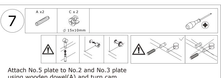
using wooden dowel(A) and turn cam lock(C) clockwise to tighten as shown.
