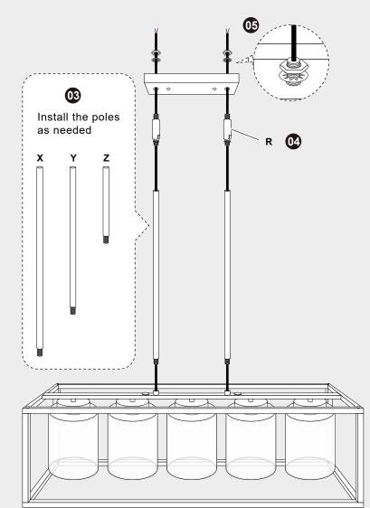
Screw the ceiling plate to the ceiling, Fixture wires should be connected to ceiling wires by color, black wire to be attached to the black wire, white to white and ground wire to ground wire.
