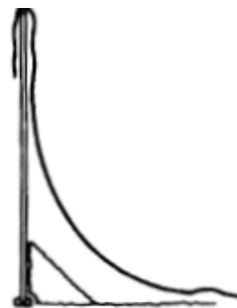
INCORRECT! DO NOT LEAVE A GAP BETWEEN LINER AND COVE. THIS WILL CAUSE DOWN- WARD PRESSURE ON THE LINER. CORRECT THIS CONDITION IF IT OCCURS.
