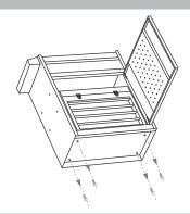
Place the cabinet on the back on a horizontal surface. Unscrew the 4 bottom screws with a screwdriver.
