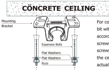
For concrete ceiling, use the percussion bit with diameter 8mm to drill holes according to the length of expansion screws. Then use the attached expansion screws to fix the hanging bracket onto the ceiling (selection is made according to actual requirements of the customers).
