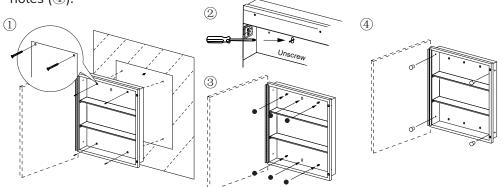
2. Cut the marked perimeter through the drywall ( $\hat{\mathbb{U}}$ ), remove the cutout ( $\hat{\mathbb{Z}}$ ), and frame the cutout opening as instructed.
