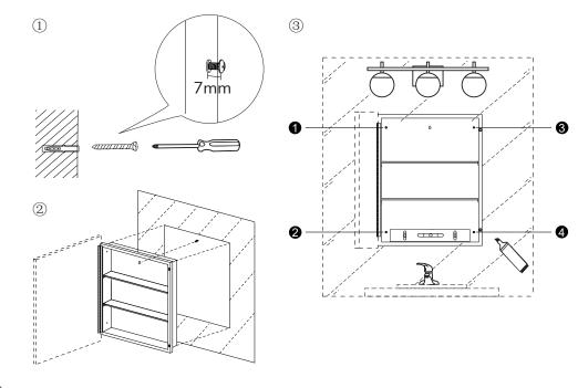
4. Put the cabinet down, punch holes at the marked spots (1) with an electric drill, then apply wall anchors with a hammer (2).
