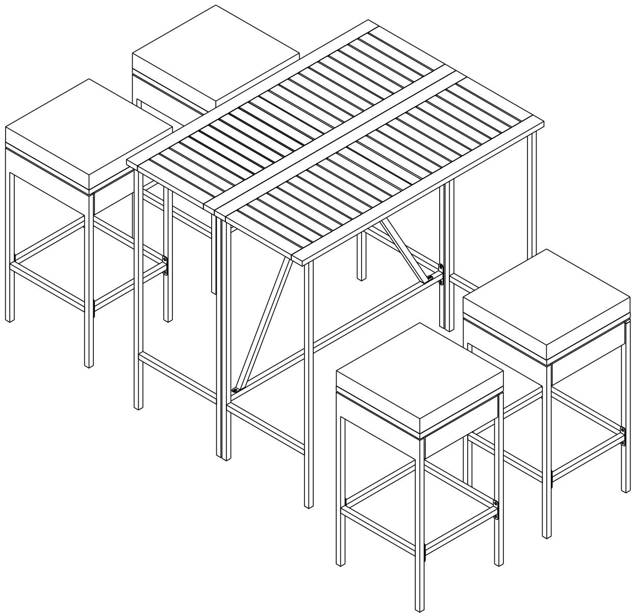
**NOTE: 50% TIGHTEN BEFORE FIXING ALL BOLTS**
