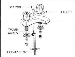
Insert lift rod down faucet hole and into holes of pop-up strap. Adjust and tighten thumb screw to obtain proper operation.
