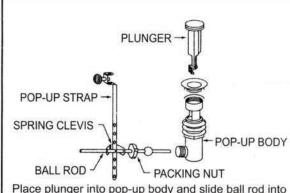
Place plunger into pop-up body and slide ball rod into plunger hole. Secure ball rod to pop-up body with packing nut.
