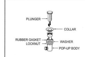
Remove collar and plunger from pop-up body. Turn locknut down as far as it will go and install washer and rubber gasket.
