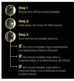
In any of these instances, it is an indication that there is an issue ON the circuit and NOT with the circuit breaker itself. (If there is no issue on the circuit to be diagnosed, tripping after a five second delay would also be a normal breaker testing operation.)
