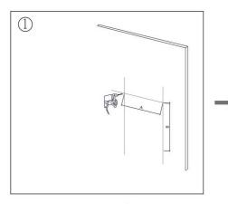
Measure the distance of the mounting hole, Drill holes with a suitable sized drill.
