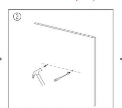
Insert the anchor and mounting screw into the wall.
