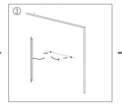
Connect the mirror wires with your main wires and hang the mounting hole to the screw on the wall.
