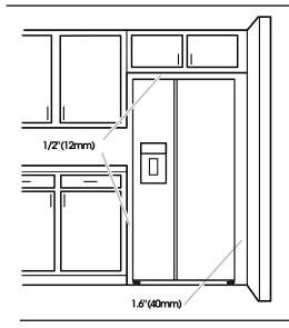
To ensure proper ventilation for your refrigerator, allow for a 1/2"(12mm) space on each side and at the top. Allow at least 2.0"(51mm) between back of cabinet and the wall. If your refrigerator has an ice maker, allow extra space at the back for the water line connections.
