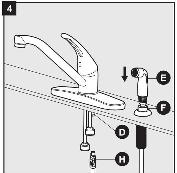
5. Connect a 1/2 in. IPS faucet connector or coupling nuts (not included) with 3/8 in. O.D. ball-nose risers (not included) to the water supplies underneath the sink using wrenches (not included).
