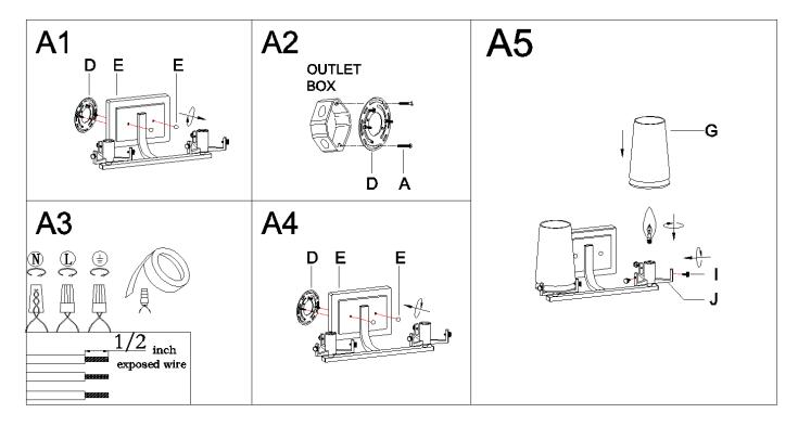
Step A1: Unscrew ball knobs (F) from back plate (E) then gently remove mounting plate (D). Step A2: Secure mounting plate (D) to the outlet box with mounting screws (A).
