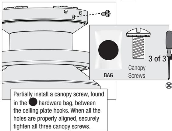
Partially install a canopy screw, found in the ● hardware bag, between the ceiling plate hooks. When all the holes are properly aligned, securely tighten all three canopy screws.
