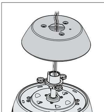
Thread the wires through the top housing. Place the top housing onto the motor housing so that the holes in the top housing line up with the holes in the motor housing and the adapter.
