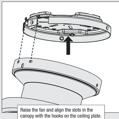
**Note:** To hang the fan, you must tilt the canopy to an almost vertical position so that the canopy slots sit on the ceiling plate hooks.
