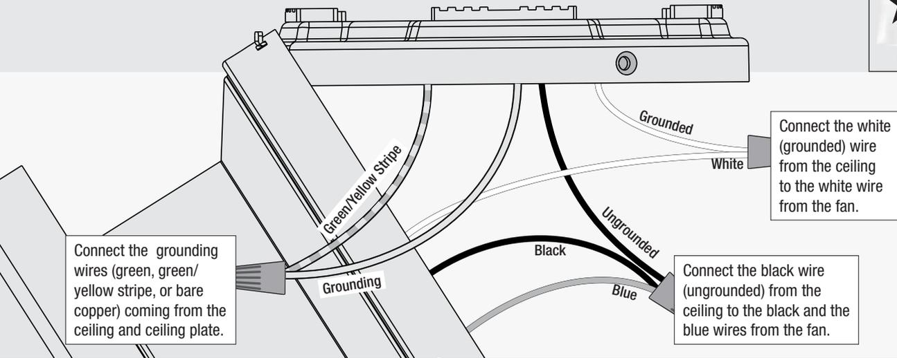
**⚠ WARNING** The ceiling fan must be grounded. If the ground wire for the installation site is not present, immediately **STOP** installation and consult a qualified electrician.
