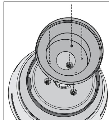
Place the canopy on the top housing. Ensure all four screw holes line up with the screw holes in both the top housing and the adapter.
