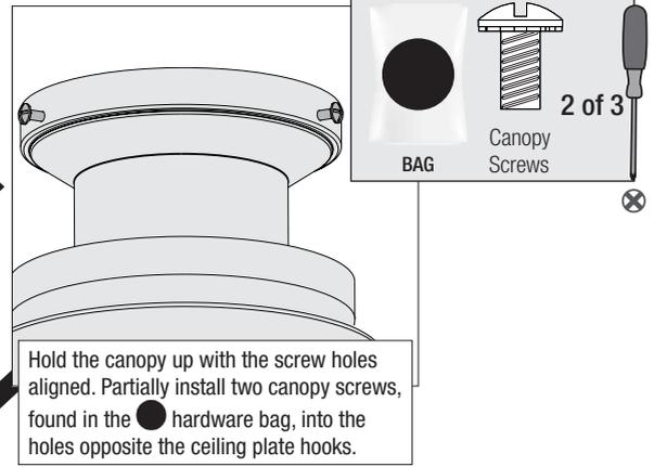
Hold the canopy up with the screw holes aligned. Partially install two canopy screws, found in the ● hardware bag, into the holes opposite the ceiling plate hooks.
