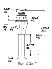
Ø1 Min to Ø1-1/2 Max. Deck Hole Openings
