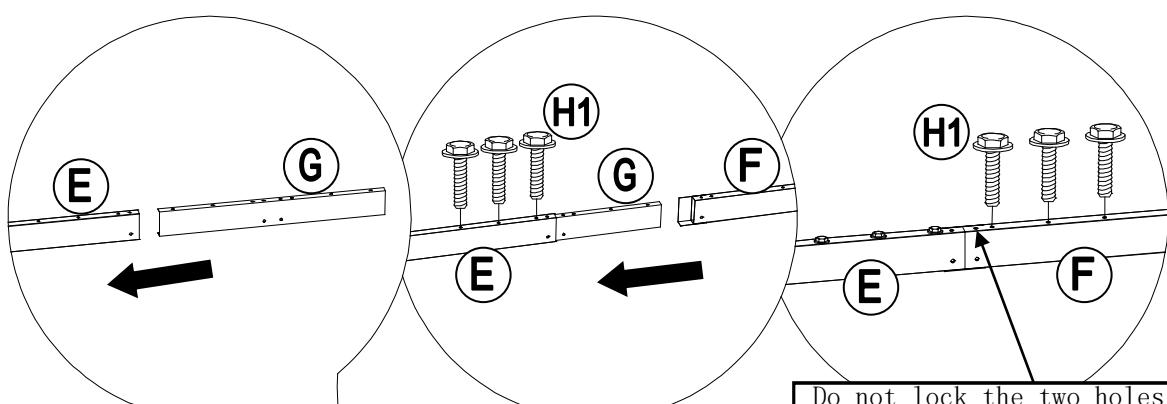
Do not lock the two holes between the long beam (E) and the long beam (F) first.
