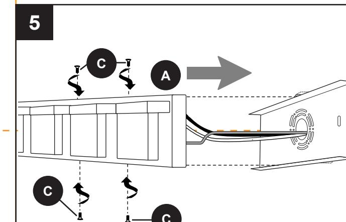
Before tightening C completely, use level (not included) to check A -- adjust if necessary.
