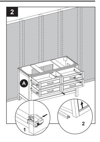
**Note:** Clean area where the vanity (A) will be permanently located prior to beginning installation, ensuring the vanity (A) will not interfere with any water supply and drain lines once mounted.
