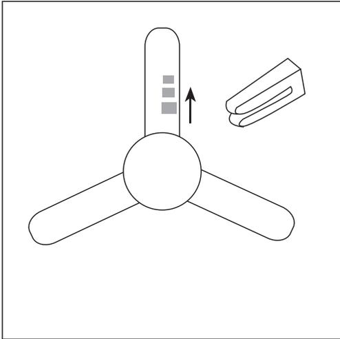
Slide the clip in small increments away from the center of that blade. Move the clip, operate the fan, then move it again until you eliminate as much wobble as possible.
