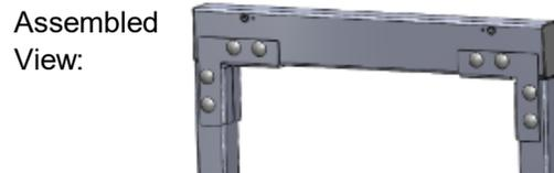
Fig 6. Attach Top Bar Assembly to Vertical Leg Assemblies.
