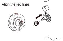
5 Use an allen wrench to tighten the HEX screw
