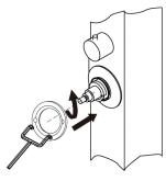
④ Press the button on the knob and put on the valve as shown ensuring the HEX screw points down
