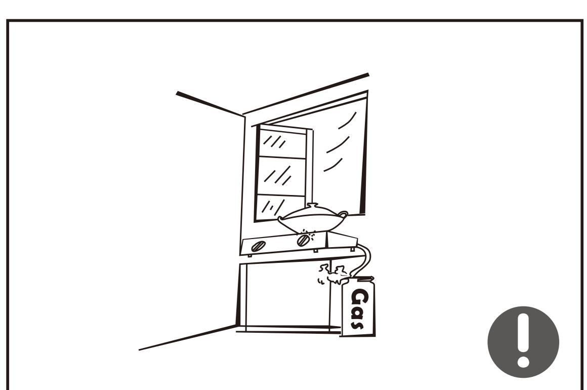
Please turn off the valve of the leaking gas and then open the doors and windows in case of leakage of gas and other flammable gases. Do not unplug the freezer and other electrical appliances considering that spark may cause a fire.
