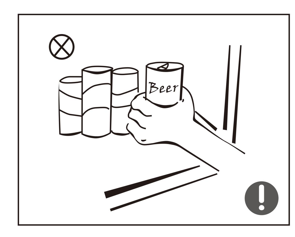
• Do not place items such as bottled or sealed container of fluid such as bottled beers and beverages in the freezer to prevent bursts and other losses.
