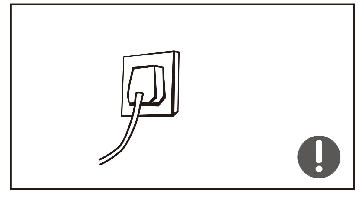
The power plug should be firmly contacted with the socket or else fires might be caused. Please ensure that the grounding electrode of the power socket is equipped with a reliable grounding line.
