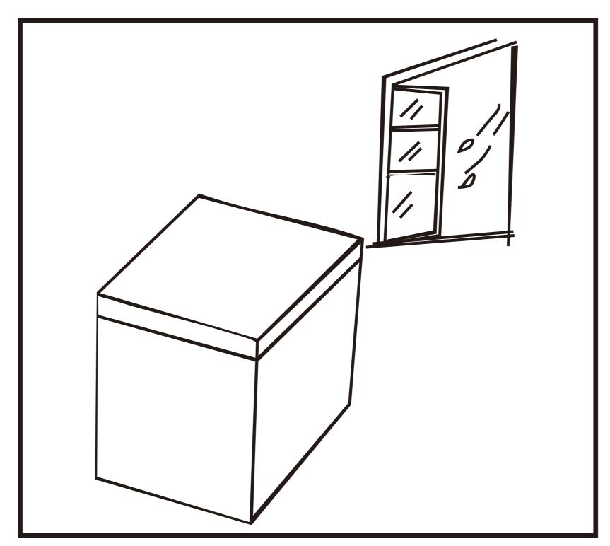
The freezer should be placed in a well-ventilated indoor place; the ground shall be flat, and sturdy.
