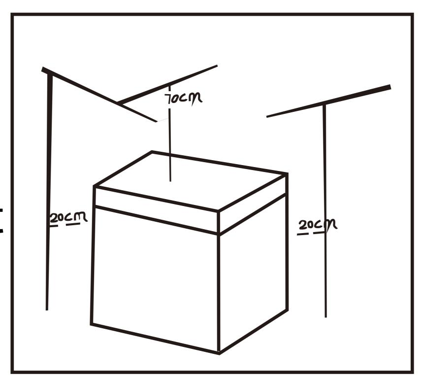
•The top space of the freezer shall be greater than 70cm, and the distances from both sides and backside shall be more than 20cm to facilitate heat dissipation.
