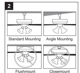
Ensure the blades (J) will be at least 30 in. from any obstructions. Also check the downrod (A) length to ensure the blades (J) will be at least 7 ft. above the floor.
