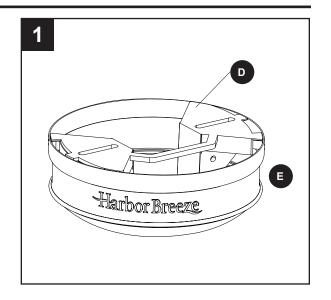
Attach mounting bracket (D) to outlet box (not included) using screws and washers provided with the outlet box.
