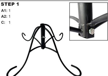
Remove Bolt and Nut (C) from Inner Leg Base (A1).
