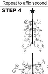
Insert assembled components from Step 2 into the base legs and secure using the wing screw on Inner Base Leg (A1).
