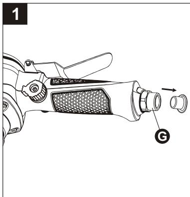
2. Add threaded sealant tape (not included) to the threading of a male plug (not included), then insert the male plug by hand into the air inlet (G). Tighten the male plug by turning it clockwise with a wrench (not included).
