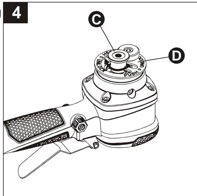
5. Push the set plate (D) forward to get the ribbed side of the set plate (D) into the hole of bearing seat (C). This ensures the bearing seat (C) is locked and stable.
