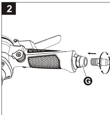
3. Place 2-3 drops of air tool oil (not provided) into the male plug before each use.
