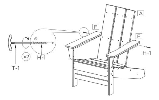
Fasten the Left Arm (E) and the Right Arm (F) to the Back Brace (A) using a Lag Screw (H-1) on either side with the 5/32" T-Handle Allen Wrench (T-1). Fully tighten all hardware from this step and all previous steps. DO NOT OVER-TIGHTEN.
