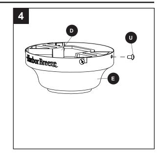
5. Attach mounting bracket (D) to outlet box (not included) using screws and washers provided with the outlet box.
