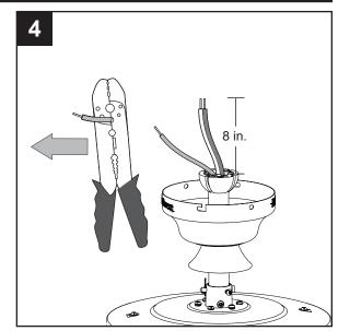
If you decided to cut back the lead wire in Step 4, strip 1/2 in. of insulation from the end of the white wire.
