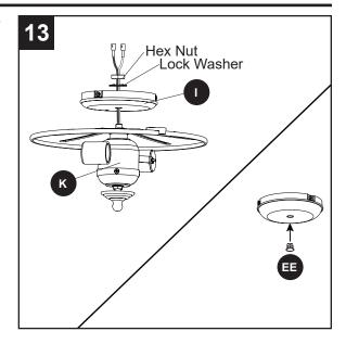
14. To install the fan without the light kit (K), remove the three switch housing screws (Z) from the switch housing cap (I). Then, attach the switch housing cap (I) to the switch housing (H) using the switch housing screws (Z). Attach the the pull chain extension (DD) to the pull chain.
