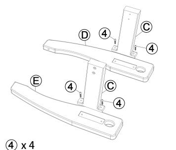
Attach "Side Frame (C)" to "Arms (D/E)" - Using "4 M6 × 30MM Bolts", tighten with Hex key.
