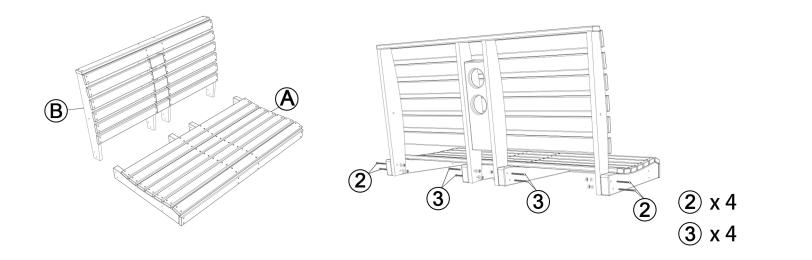
• Attach "Back (B)" to "Seat (A)" - Using "2 M6 × 60MM Bolts" and "3 M6 × 50MM Bolts", tighten with hex key and wrench.
