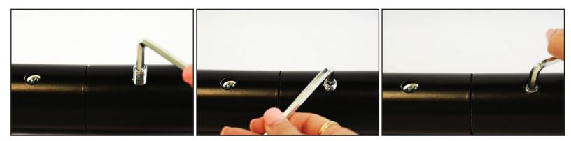
Using the hex wrench, continue to tighten until headless set screw is <u>very tight</u> and resistance is felt. Then, tighten another rotation to ensure the expansion joiner is locked.
