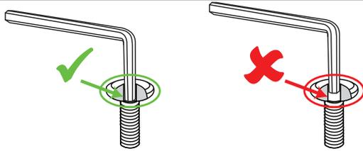
**Tip:** Always fully insert the hex key inside the designated notch of the bolt. If the hex key is not entirely inside the notch, the hex key could slip out, causing damage to the bolt head. In addition, repeated hex key slipping will cause the notch to become rounded, making it difficult or impossible to tighten the bolt.
