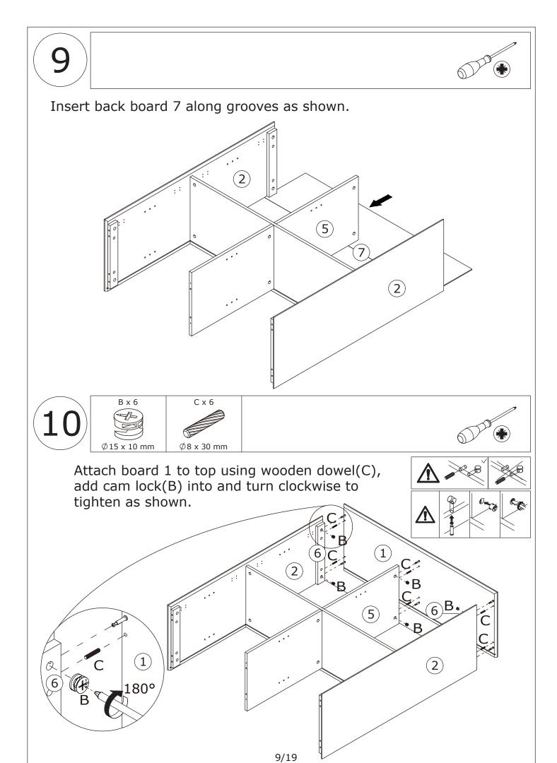
Insert back board 7 along grooves as shown.
