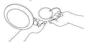
2a Align the torsion springs to the housing and press the fixture flush to the ceiling. Squeeze torsion springs together and install into torsion spring brackets inside recessed housings and press the fixture flush to the ceiling.
