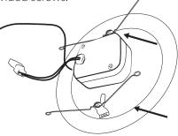
Disconnect Edison base from downlight and screw into socket inside recessed housing. (GU24 base option available). (Base not needed if using NICOR 17014A-LED-ID)
