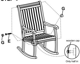
Invert the rocker and repeate the step 3 procedure to secure using 1 1/4" bolts (E).
