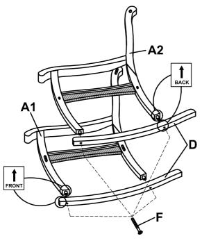
Attach each rocker (D) to right and left side frame (A1 & A2) as picture shown, connecting front of rockers to front legs first then the back of rockers. Secure connections with 1 3/4" bolt (F).
