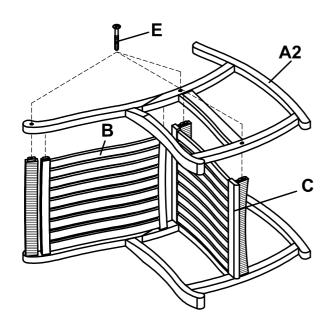
Attach the leftt side frame (A2) onto Head back support (B1), Back support(B2) and seat (C). Secure using 1 1/4" bolts (E), as shown.
