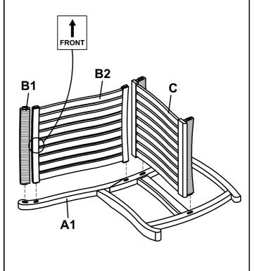
Install Head back support (B1), Bask support (B2) and seat (C) into corresponding holes of left side frame (A1).
