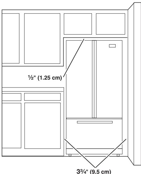
To ensure proper ventilation for your refrigerator, allow for a 1/2" (1.25 cm) space at the top and behind the refrigerator. If your refrigerator has an ice maker, allow extra space at the back for the water line connections. When installing your refrigerator next to a fixed wall, leave a 3-3/4" (9.5 cm) minimum space between the refrigerator and wall to allow the door to swing open.
