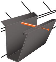
**Spike & Ferrule** Insert ferrule into gutter lined up with a rafter, hammer spike through gutter and drip edge into the fascia.
