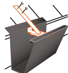
**Strap Hanger** Hook the hanger under the front lip of the gutter. Carefully lift shingles then nail into the roof deck.
