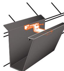
**Hidden Hanger** Hook the hanger under the front lip of the gutter. Drive a nail or screw through the hole in the hanger into the fascia.
