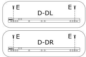
Fix runner(D-DL) and (D-DR) to board 16 and 15 with screw(E) as shown.
